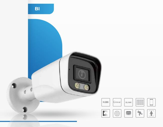
Human detection IP camera, adopt Ingenic 22nm chip,built-in Al algorithm, H.265 / H.264 Compression format, D-WDR, 3D DNR, 3.6/4mm lens is optional, 2 pcs IR lights, IR distance 20M
